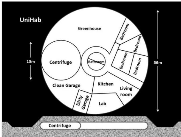
**Figure 4.** Simple illustration of a large inflatable habitat covered by regolith for shielding and with an indoor centrifuge.
