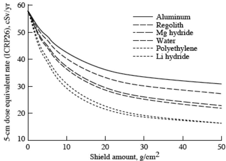
**Figure 3.** GCR exposure versus depth of various materials [Simonsen et al. 1997]
